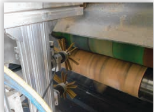
Trim Removal System installed on a Flexo-Folder-Gluer
