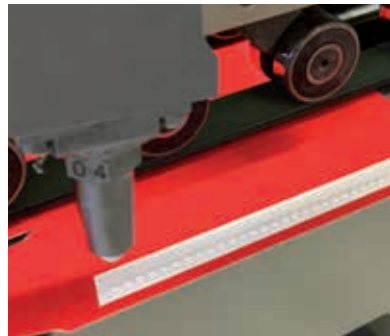
ERO glue guns apply precise glue dot patterns, allowing important glue savings
