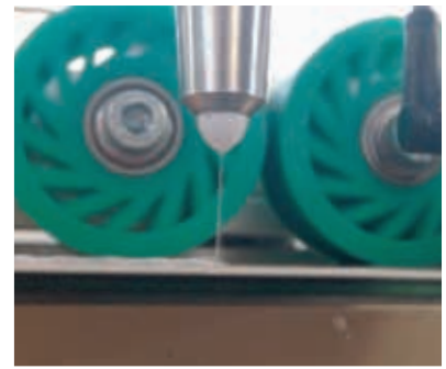
Ceramic stem spheres and nozzles guarantee a longer life time
