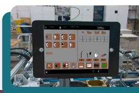
ERO uses an iPad as upgrade to traditional control panels. Lightweight, intuitive and convenient, iPads allow independent monitoring from any place.
